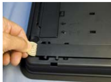
Fig 2a - Lifting out the Legs
